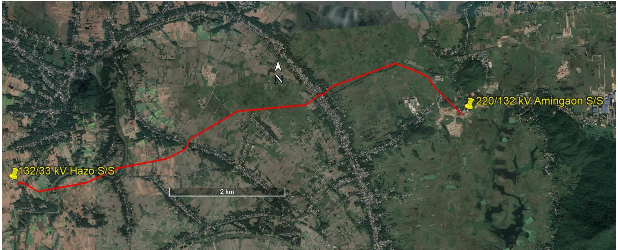
Figure 4.2: Satellite Imagery Showing Route of Amingaon (new) – Hazo (new) 132 kV D/C Line
