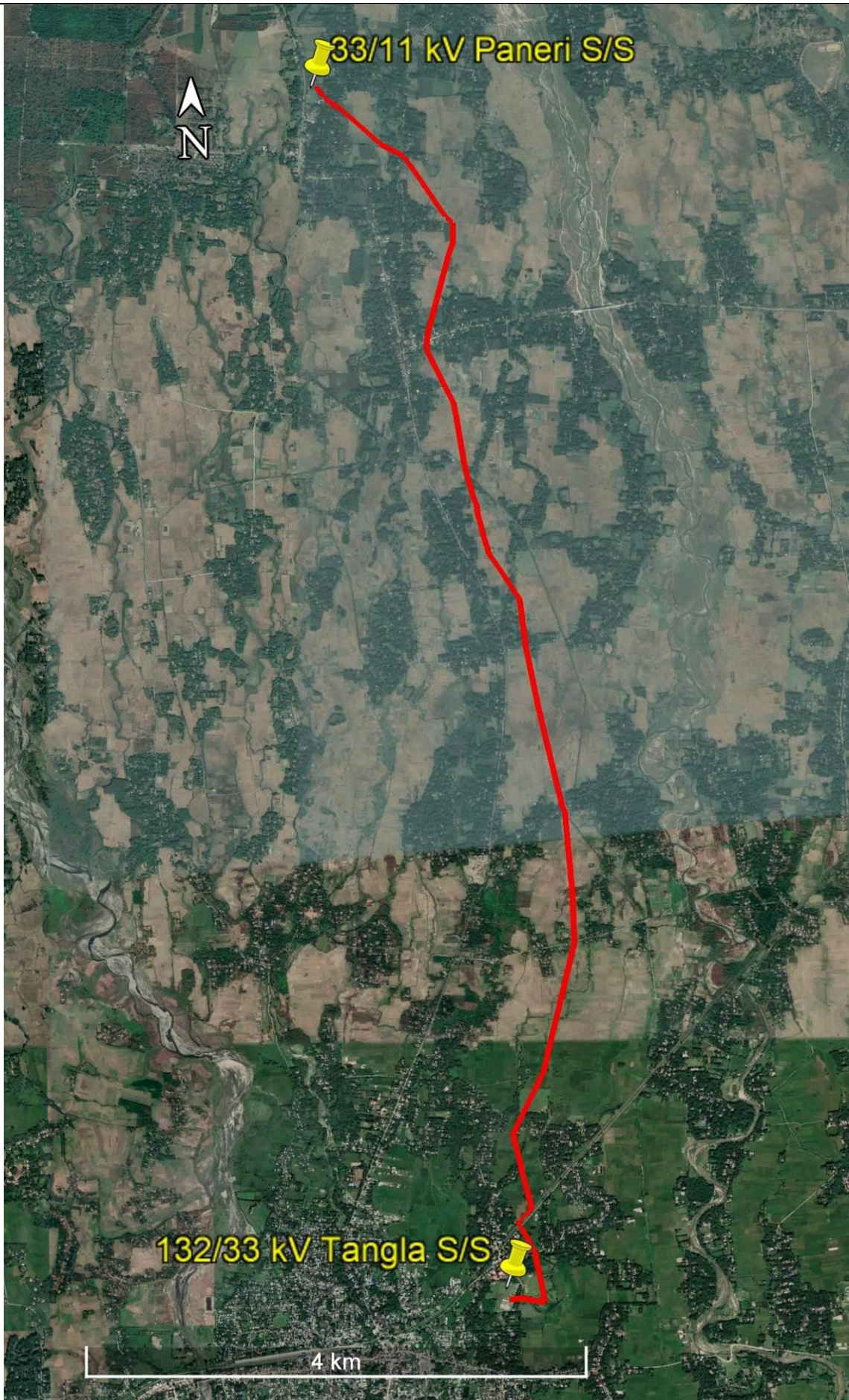
Figure 4.12: Satellite Imagery Showing Route of 33 kV line from 132/33 kV Tangla (new) S/S to 33/11 kV Paneri (existing) S/S
