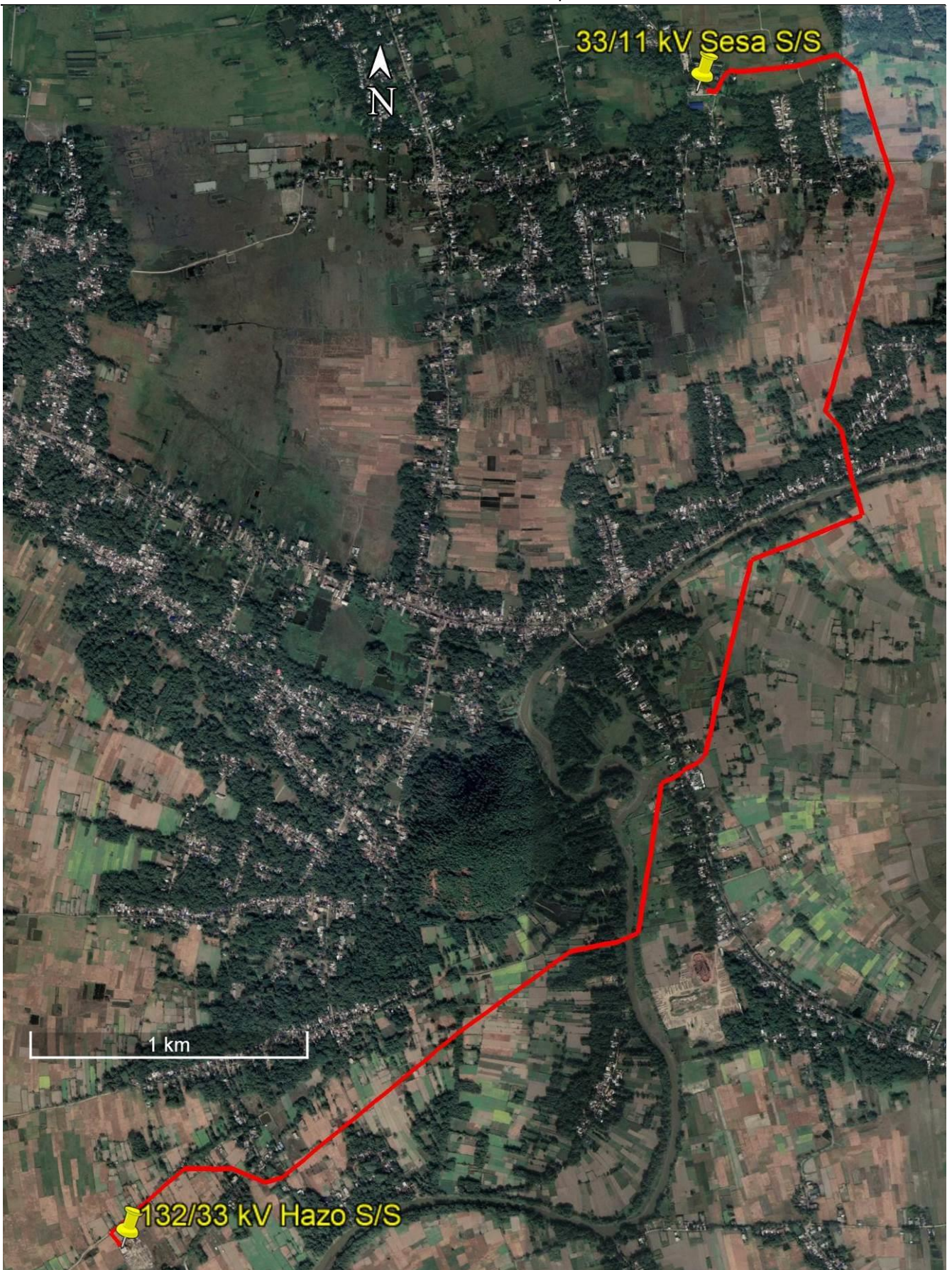
Figure 4.8: Satellite Imagery Showing Route of 33 kV line from 132/33 kV Hazo (new) S/S to 33/11 kV Sesa (new) S/S
